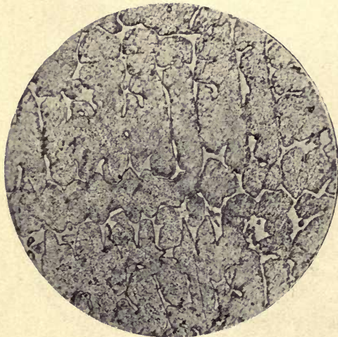
Fig. 17. \times 450 Alloy 23. Cu 77.2 Sn 5.6 Zn 22.2. Annealed at 450° C. \alpha + \gamma .
